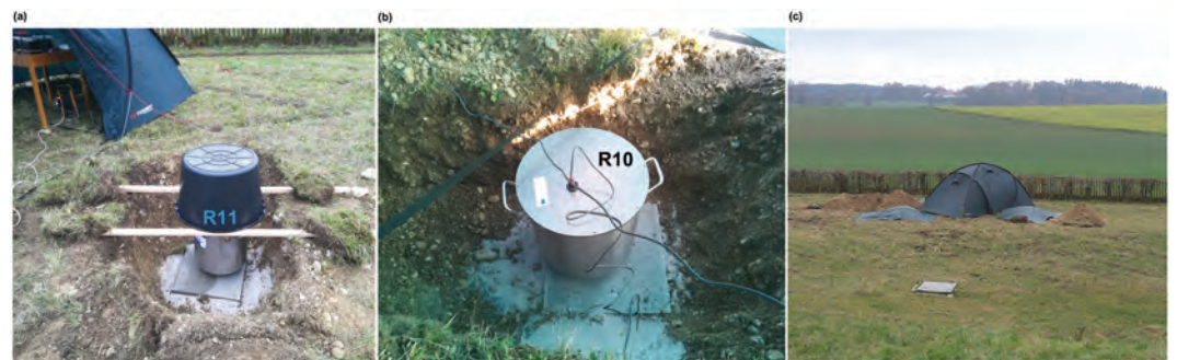
Figure 6. Field deployment of the Rotaphones-CY involved in the Geophysical Observatory in Fürstenfeldbruck (GOF) experiment: (a) Rotaphone R11, NW apex of the triangular array, before the waterproof foil was laid over, (b) the central Rotaphone R10, sheltered by a tent, and (c) the whole array as viewed from the North, R10 inside the tent, R8 and R11 on both sides, R13 hidden behind the tent.
